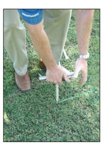
Disengage tool from sensor with ejector button.
