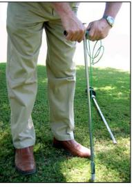
Sensor is placed on end of #1017 Insertion Tool.
