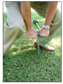
Use tee handle to "seat" sensor in bottom of hole, maximum depth is 30" (76 cm).
